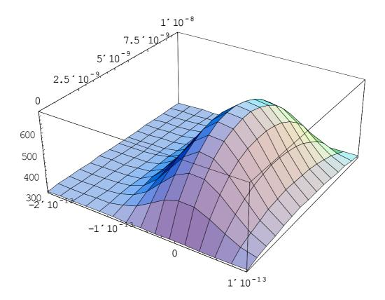
Figure1: The temperature variation versus time and spatial dimension in gold-chromium two layer film.(500  $A^0$  gold , 500  $A^0$  chromium)
