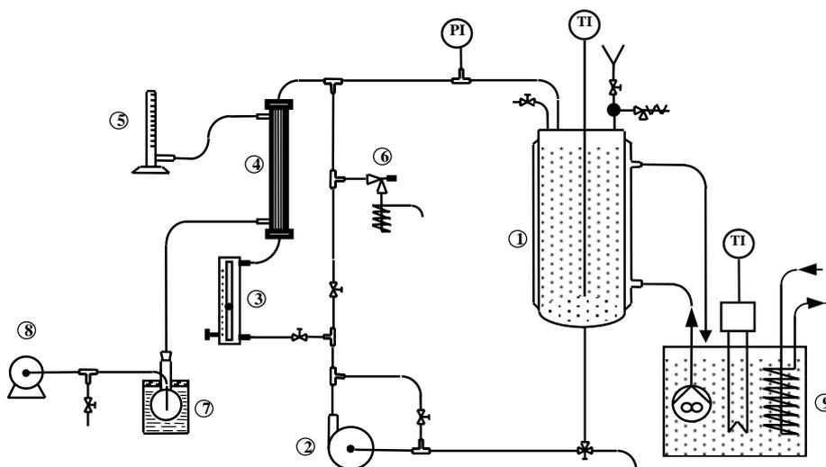
1 - Feed vessel 2 - Feed pump 3 - Flowmeter 4 - Hollow fiber module 5 - Vacuum gauge
