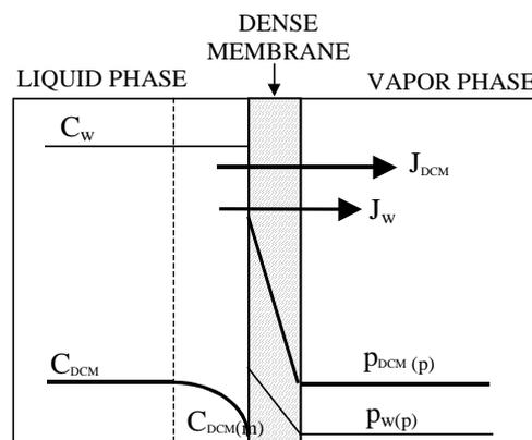
Figure 1. Diagram of concentration gradients in a three phase pervaporation system
