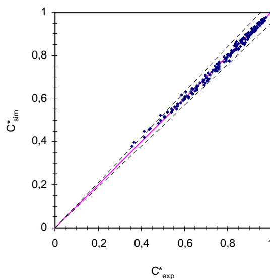
Figure 5. Parity graph of simulated dichloromethane concentration vs. experimental dichloromethane concentration.
