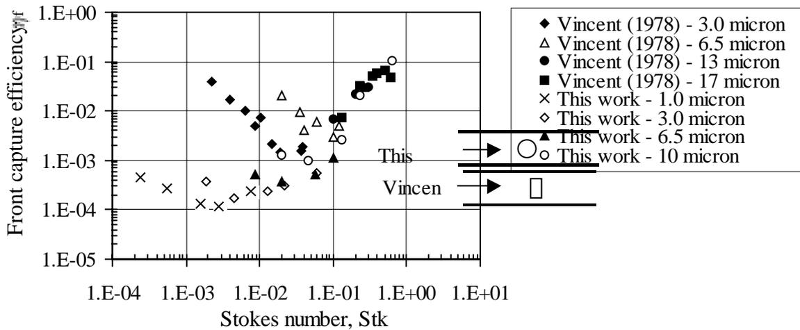
**Figure 1** Capture efficiency as a function of Stokes number
