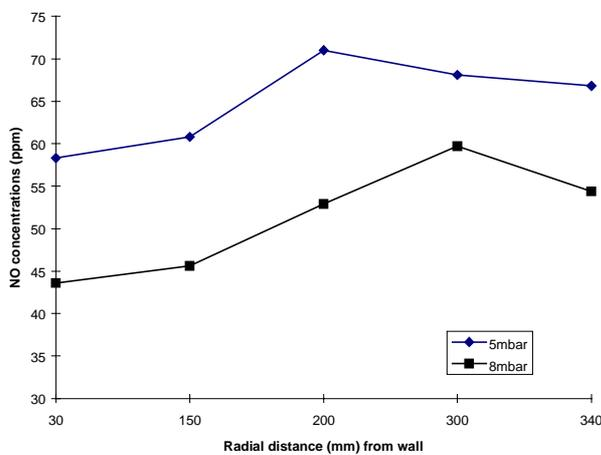
Figure 4: NO profile at rear port, steady state, 825kW, 5mbar air inlet pressure.
