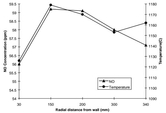
Figure 2c: NO and Temperature profile, steady state, 825kW, 8 mbar air inlet pressure, port 3.
