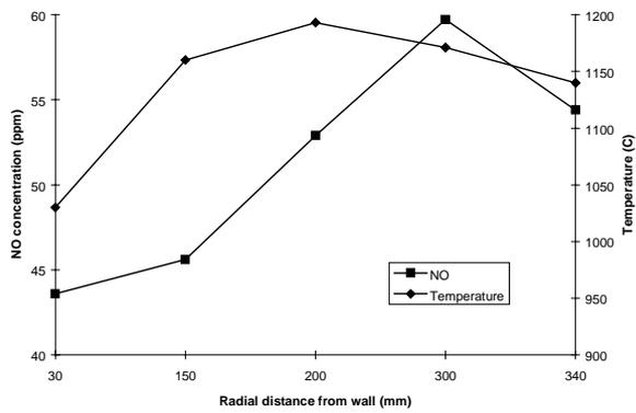
Figure 2b : NO and Temperature profile, steady state, 825kW, 8 mbar air inlet pressure, port 2.
