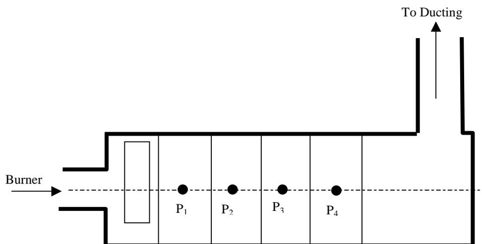
Figure 1: Schematically Stainless steel cylindrical ceramic line tunnel furnace
