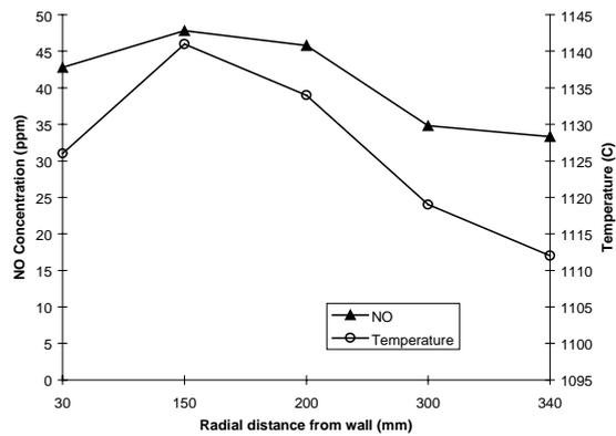
Figure 2d: NO and Temperature profile, steady state, 825kW, 8 mbar air inlet pressure, port 4.
