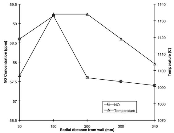
Figure 3: NO concentration, steady state, port 1, 5mbar and 8 mbar.
