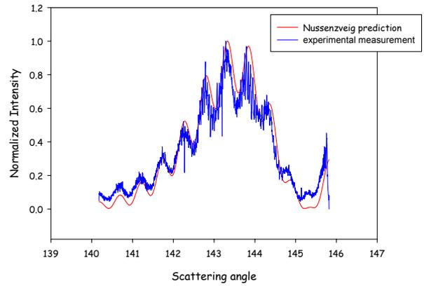
Figure 3: a couple of experimental rainbow signal, with the best fitting by Nussenzweig theory.
