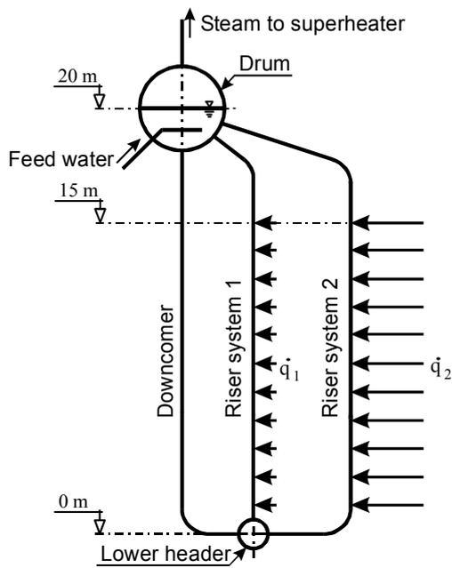
Figure 1: Two-pass boiler
