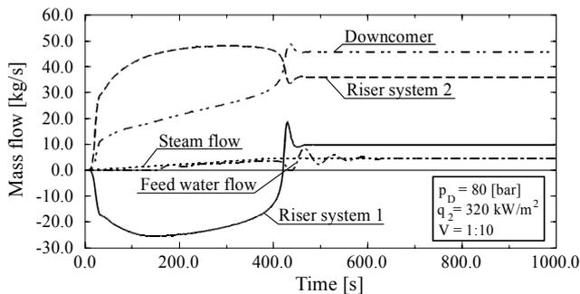
Figure 3: Mass flow in the tubes of the two-pass boiler ( $V=10$ )
