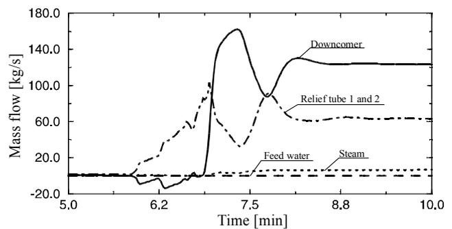
Figure 6: Mass flow in the tubes of the HRSG
