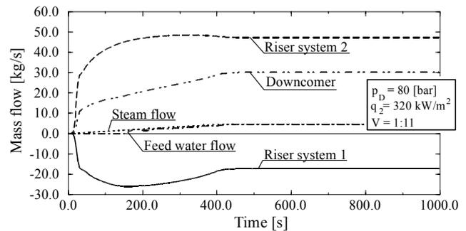
Figure 4: Mass flow in the tubes of the two-pass boiler ( $V=11$ )
