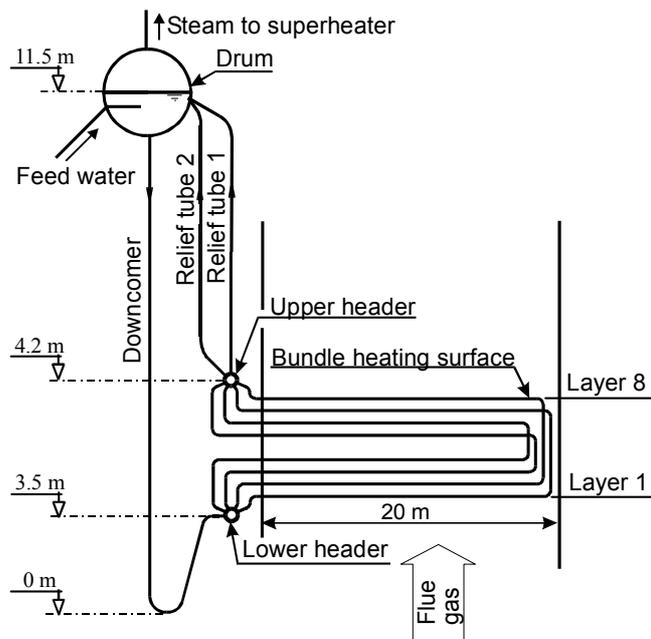
Figure 2: HRSG with a horizontal tube bank
