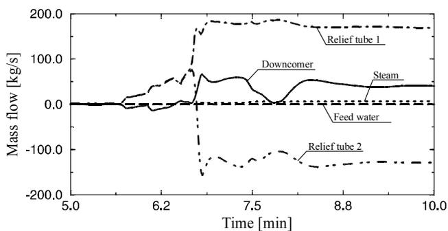
Figure 5: Mass flow in the tubes of the HRSG
