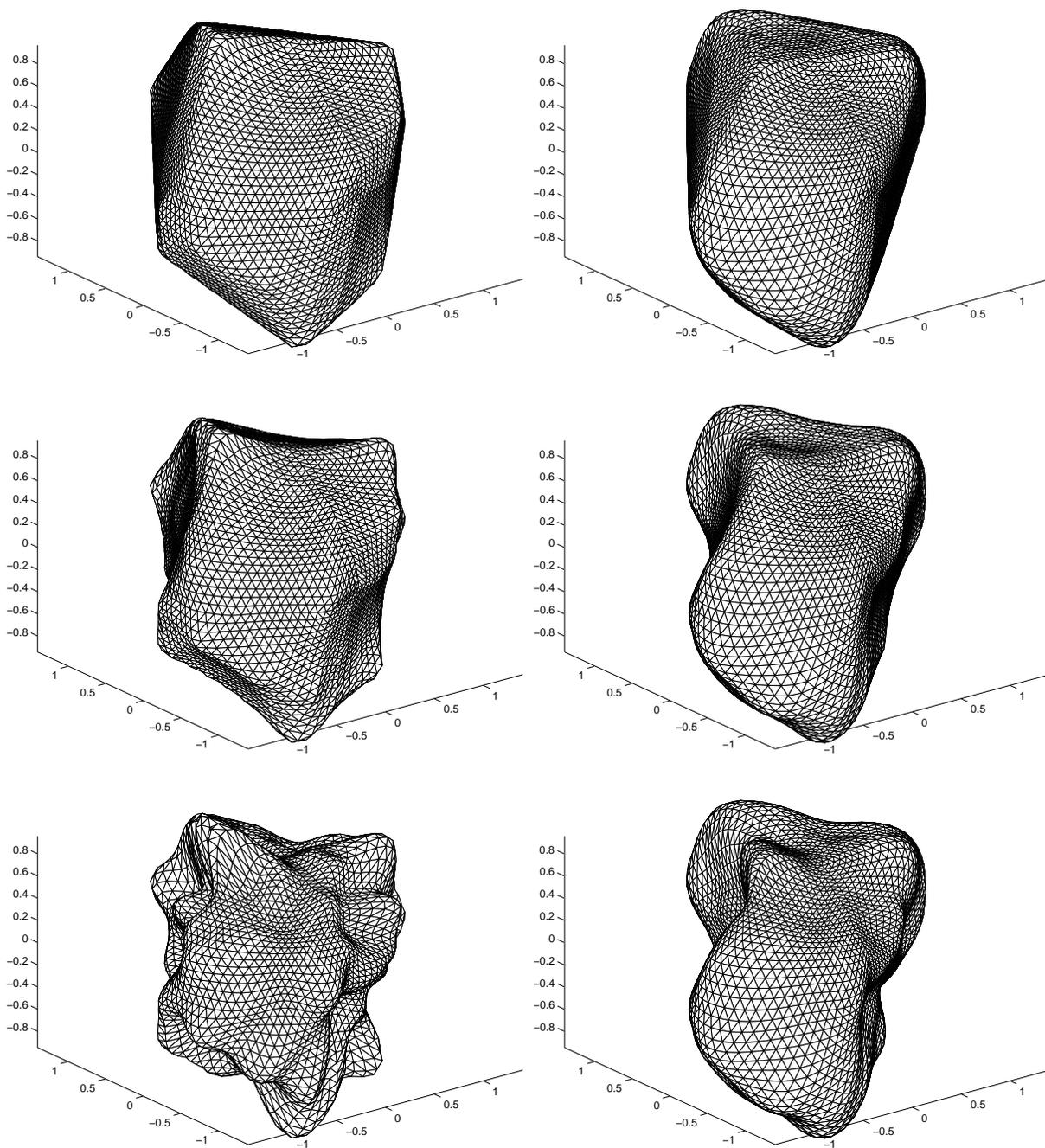
Figure 1: Example shapes corresponding to the Gaussian-random-sphere radial-distance standard deviations and covariance-function power-law indices  $\sigma = 0.2$  and  $\nu = 2$  (left) as well as  $\sigma = 0.3$  and  $\nu = 4$  (right). We show the original shapes (bottom;  $h = 0$ ) and their concave hulls generated with spheres of scale radii  $h = 2$  (middle) and  $h = 2 \cdot 10^4$  (top).
