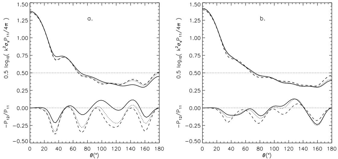
Figure 3: Discrete-dipole scattering-phase-matrix elements  $k^2\sigma_s P_{11}/(4\pi)$  (top;  $\sigma_s$  is the scattering cross section) and  $-P_{12}/P_{11}$  (bottom) for the particles left and right in Fig. 1 for the equal-volume size parameter  $x_{ev} = 5$  and refractive index  $m = 1.55 + i10^{-4}$ . The solid, dotted, and dashed lines refer to the bottom, middle, and top particle geometries in Fig. 1, respectively.
