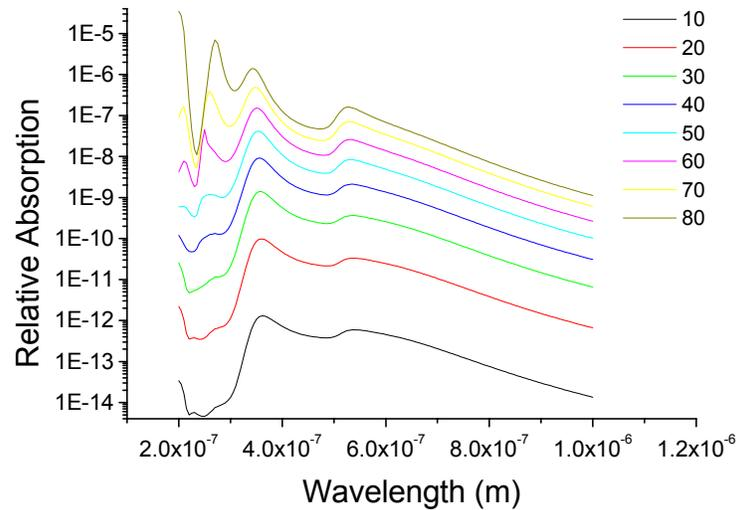
Figure 1: Spectral absorption of surface plasmon waves by gold particles, 10-80 nm in diameter. The numbers in inset corresponds to particle diameters, in nm.
