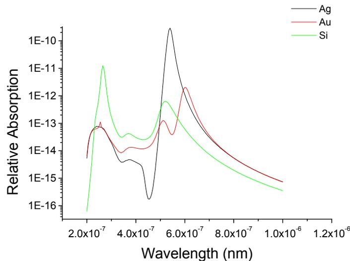
Figure 2: Spectral absorption of surface plasmon waves by gold particles, with a gold, silver or silicon probe 10 nm above the particle. Particles are 10 nm in diameter.
