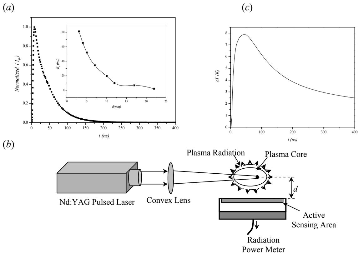
Figure 1(a). The intensity profile of the LIP approximated by normalizing the laser induced-optical emission in time ( $t$ ) measured by [5]. The radiation energy obtained at various gap distances is plotted in the inset, (b) schematic of the LIP radiation energy measurement experimental setup and (c) the transient temperature profile on the surface of the chromium film subjected to nanosecond impulsive radiation of LIP.
